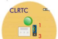
Figure 3 - 1 : Clear CMOS Jumper
